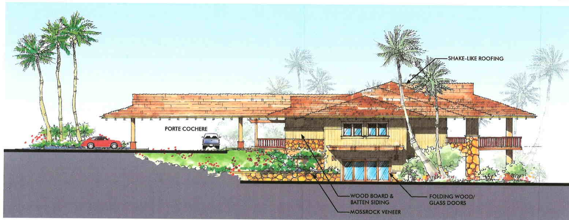
New Lobby Building Side Elevation
