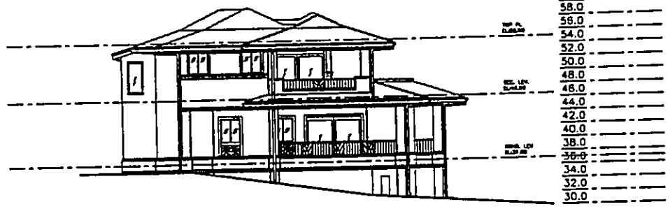
DWELLING - RIGHT SIDE ELEVATIONS SCALE: 1" = 20'
