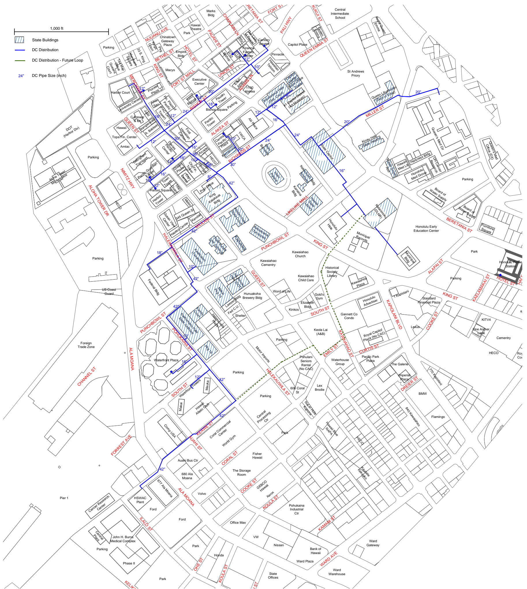
Figure 2-14: Distribution System Route and Pipe Sizes
