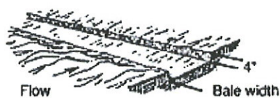
Figure 3: Constructing a straw bale barrier to slow runoff and prevent erosion.
