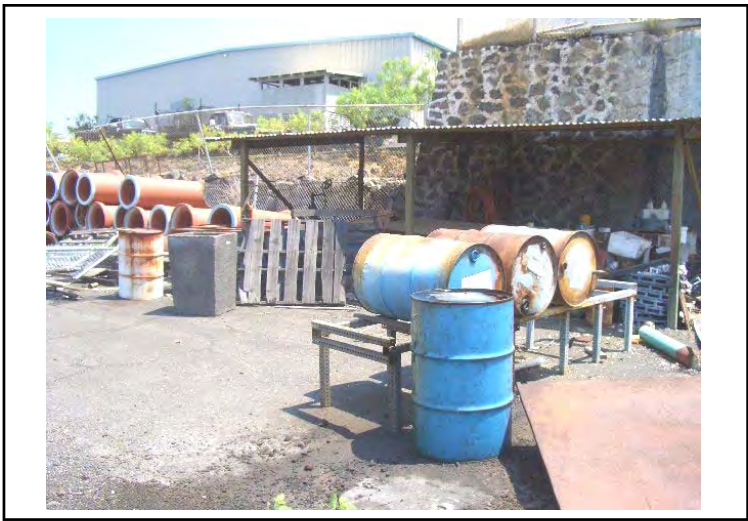
Photograph 5. A view of the 55-gallon drums containing used oil. The drums were in poor condition; however no leaks or stains were observed (May 13, 2007).
