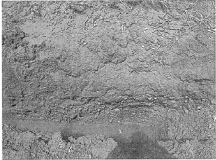
Figure 22 Test Trench 2, West Stratigraphic Profile Showing Strata I, II and III. Note River Cobbles above Water Table.
