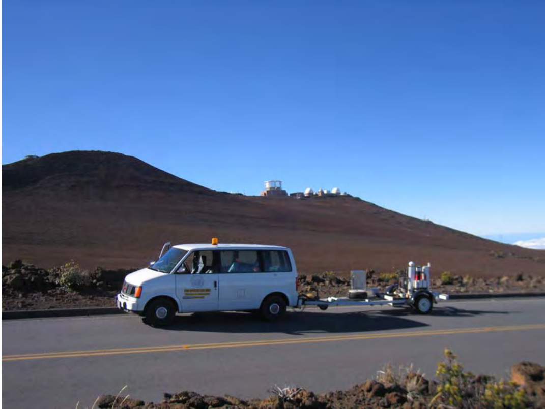
Photo 20 ---MP- 20.4, FWD testing in the uphill lane
