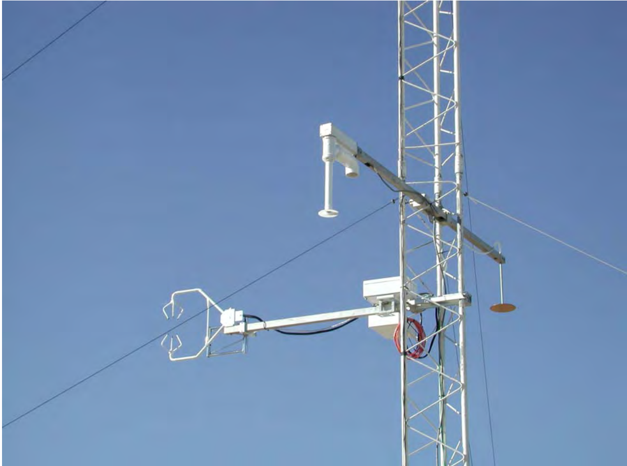
Figure 9.6: Sensors (hygrometers and sonic anemometers) mounted on a tower in Erie, Colorado for in-situ measurements of C_n^2 . These estimates are used to verify the ATST seeing analysis.
