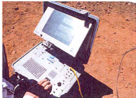
Fig. 3 - Freedom Data PC for SASW Surveys
