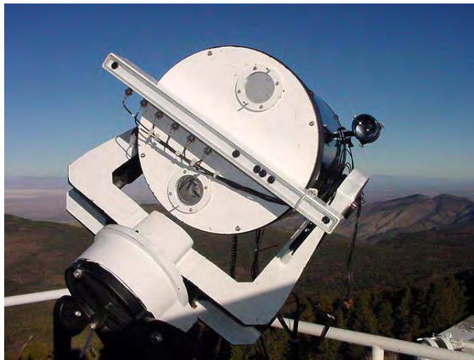
Figure 8.1 – The ATST seeing monitor. Visible are the two circular apertures for the S-DIMM, the linear array of six scintillometers for the SHABAR, and the Meade telescope.
