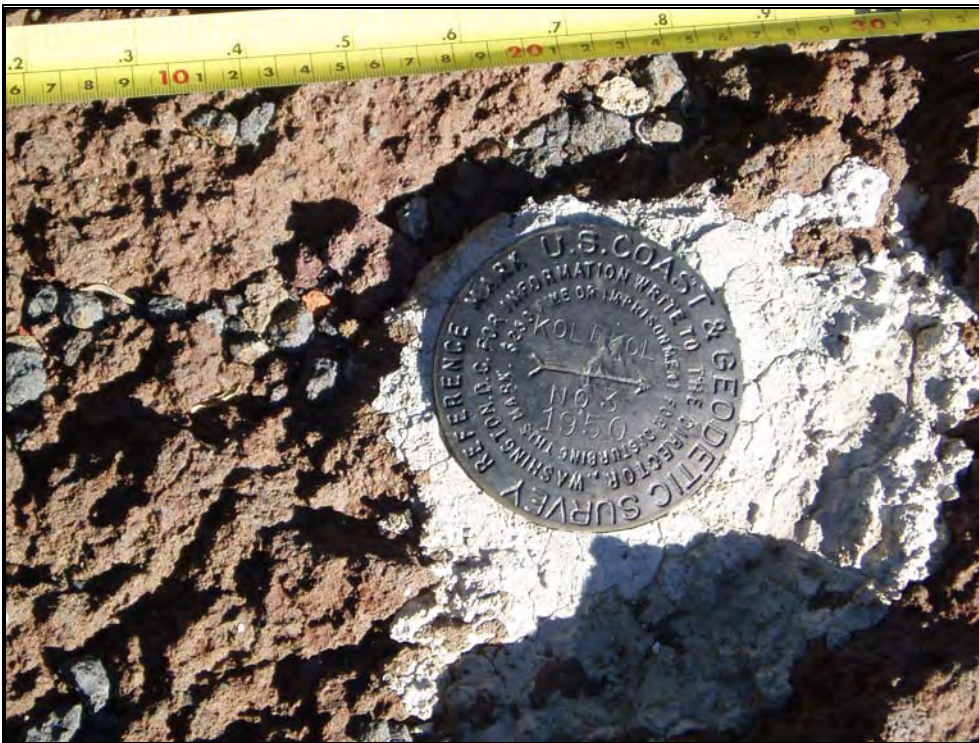
Photograph 5: View of a Reference Mark—US Coast & Geodetic Survey disc (dated 1950).
