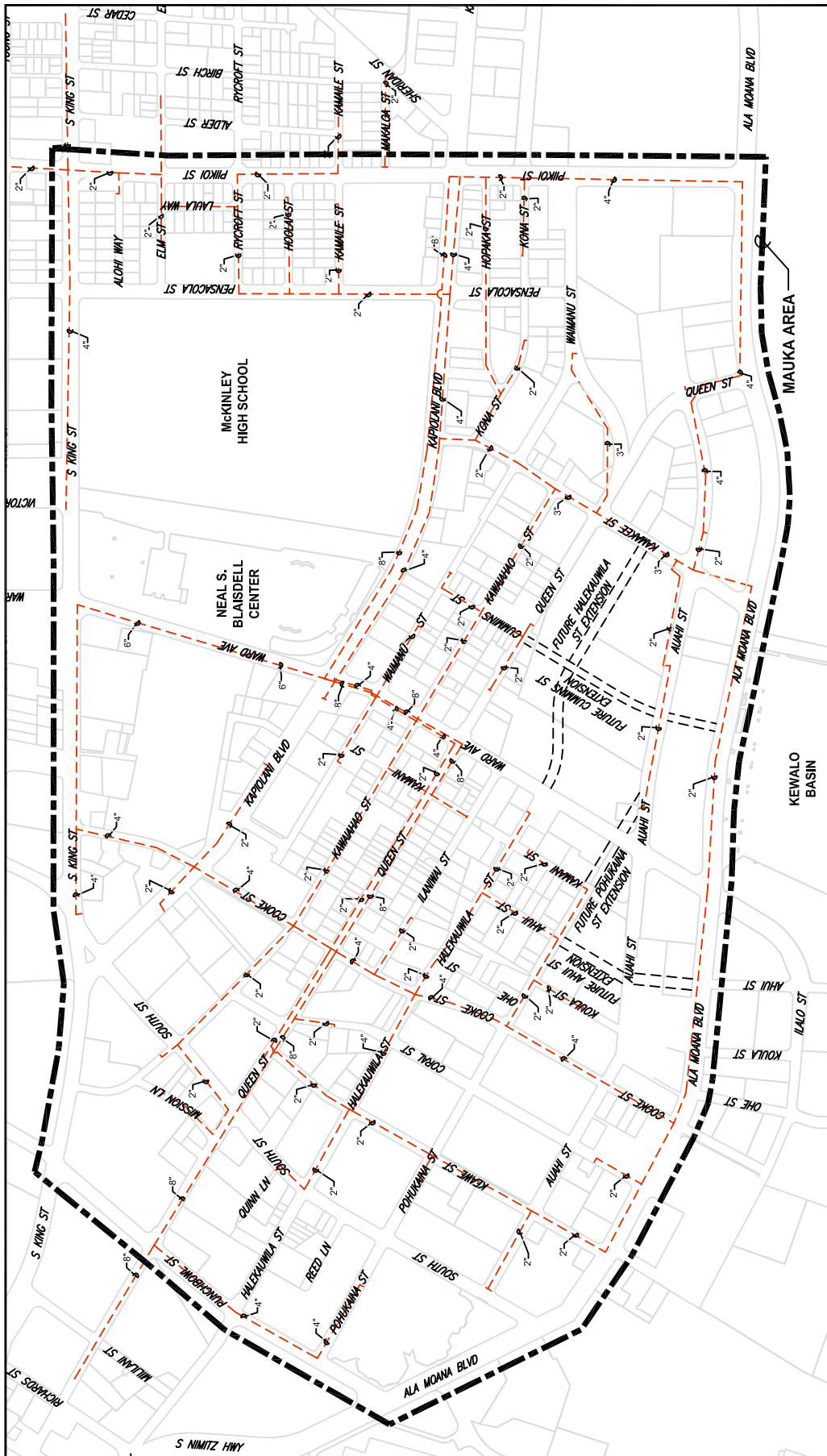
Figure 7 - Existing Synthetic Natural Gas Systems
