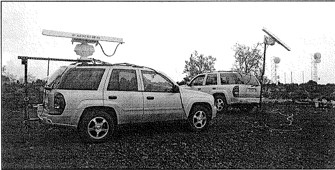
Figure 5. Furuno Model FR-1500 Mark 3 mounted on 4x4 vehicles at the proposed 'Ānuenue radio relay tower site, Ka'ūpūlehu, Hawai'i.
