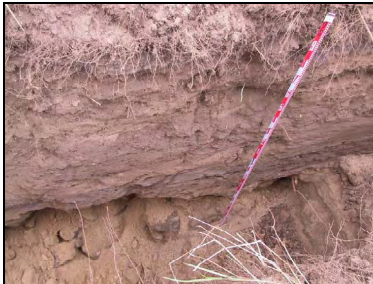
Figure 19. Photograph of the south profile of Trench 7 showing sand layers, note high energy sand and boulder layer at the base of the excavation
