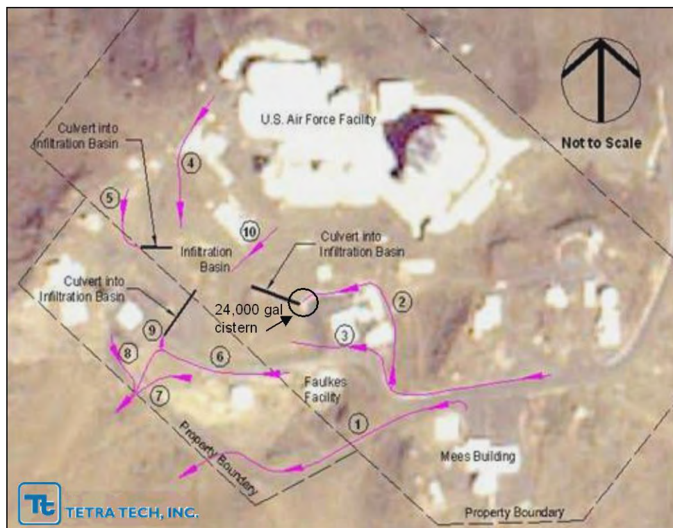
Figure 2-10 Existing Stormwater Runoff Patterns at HO
