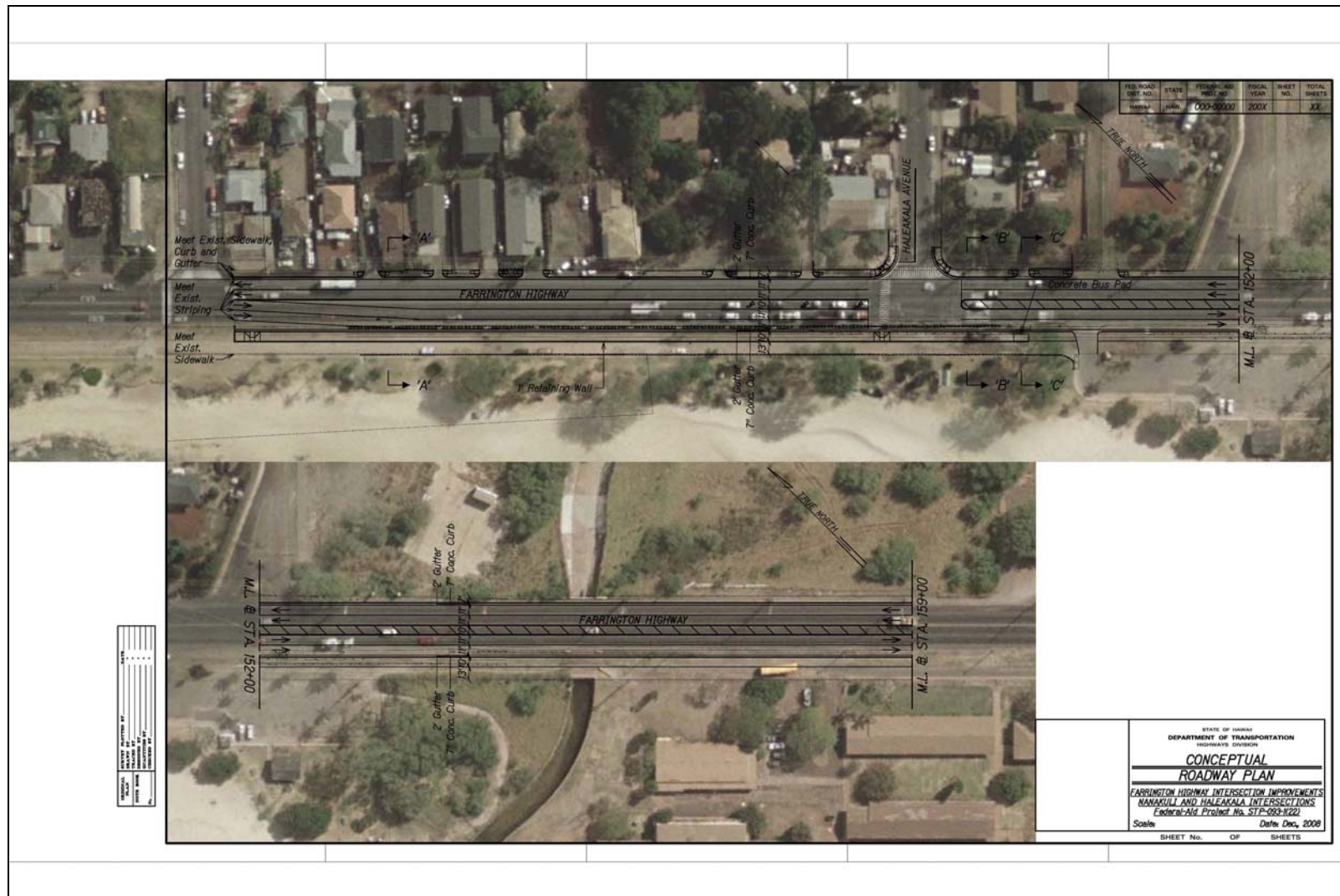
Figure 6. Conceptual Roadway Plan overlain on an aerial photograph, north portion, showing vicinity of Farrington Highway and Helelua Street (HDOT 2008)
