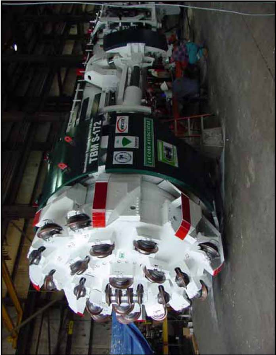
Rock Boring TBM with Rotating Cutter Head
