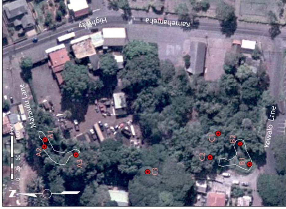
Figure 5. Aerial (satellite) image of Project area with soil pit locations (red dots) and approximate boundaries (thin white lines) of wetlands A and B.
