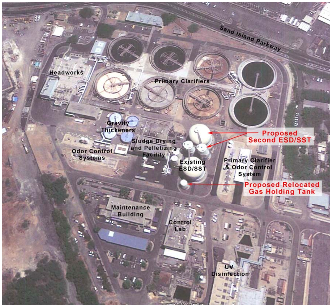
Figure 2-5, Aerial View of Sand Island WWTTP with Simulated Rendering of Proposed Second ESD/SST.
