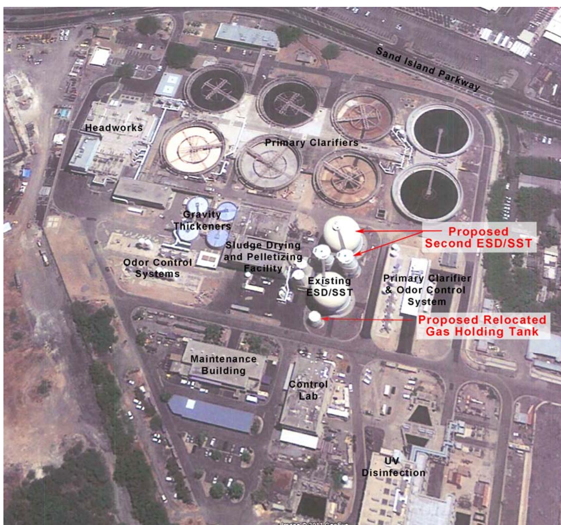
Figure 2-5, Aerial View of Sand Island WWTTP with Simulated Rendering of Proposed Second ESD/SST.
