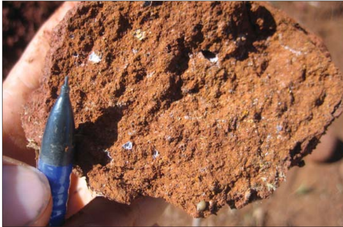
Figure 5: Detail photograph of deteriorating bedrock from Context 3, showing mineral phenocrysts and vesicles in groundmass. This piece is from Trench 8. It is likely to have been a piece of the Kōloa series basanite, and the remaining mineral phenocrysts are likely to have once been olivine. The tip of a mechanical pencil is included for scale.
