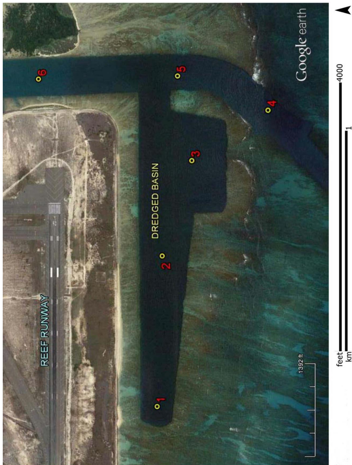
FIGURE 1. Aerial image of basin dredged in reef off the Reef Runway on the south shore of Oahu, Hawaii. Yellow circles show locations of six water sampling stations within the dredged basin and channel leading from Keehi Lagoon to the open ocean. See Table 1 for coordinates of sampling locations.
