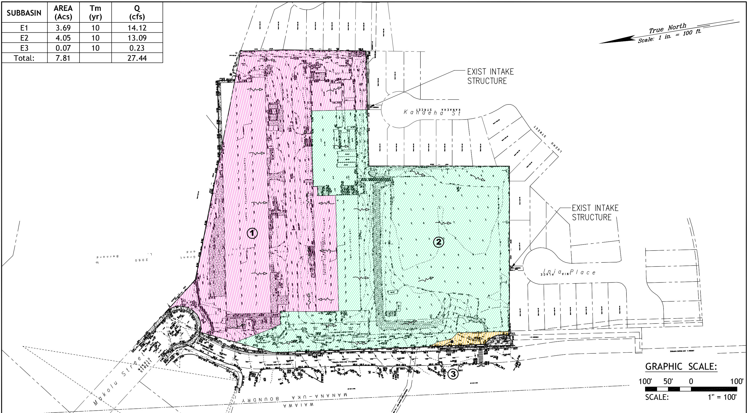
MANANA CORPORATION YARD PEARL CITY, OAHU, HAWAII EXISTING DRAINAGE CONDITION
