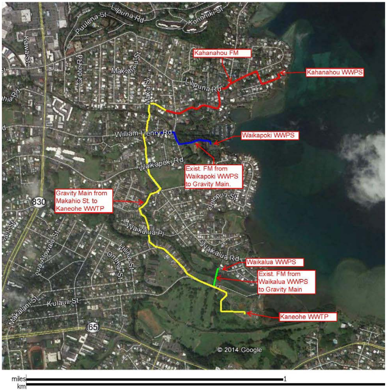
Figure 2-4: Overall Sewer System to Kaneohe WWTP
