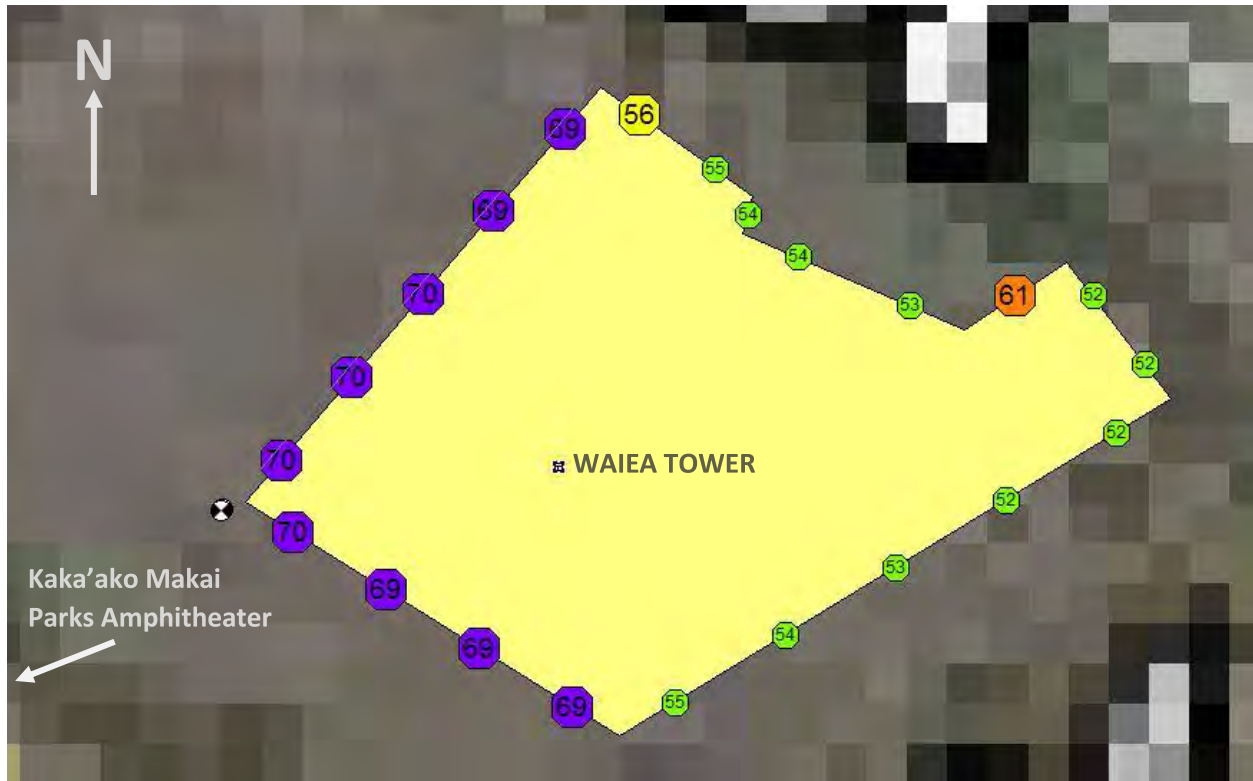
Figure 10. Amphitheater Sound Levels at the Waiea Tower Building Facades (Kona Winds)
