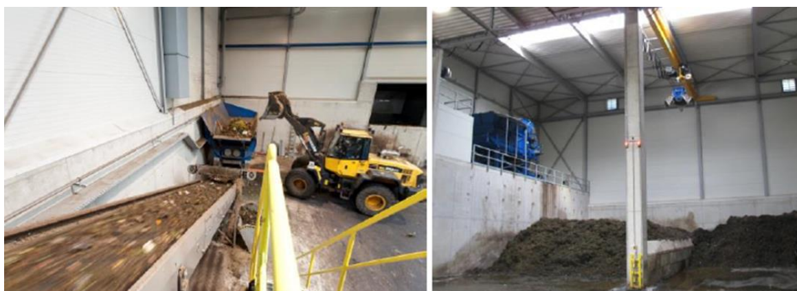
Figure 3-6: Photo on left shows loader infeed; photo on right shows automatic crane delivery.
