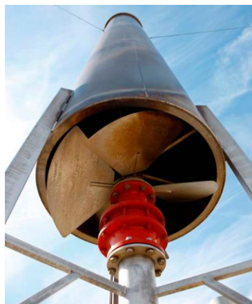
Figure 3-10: An example of the emergency flare configuration
