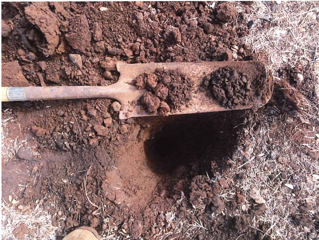
Sampling Point 5B. Dark reddish-brown silt loam over dark reddish-gray clay loam. Saturation at 17 inches. Water table at 20 inches.
