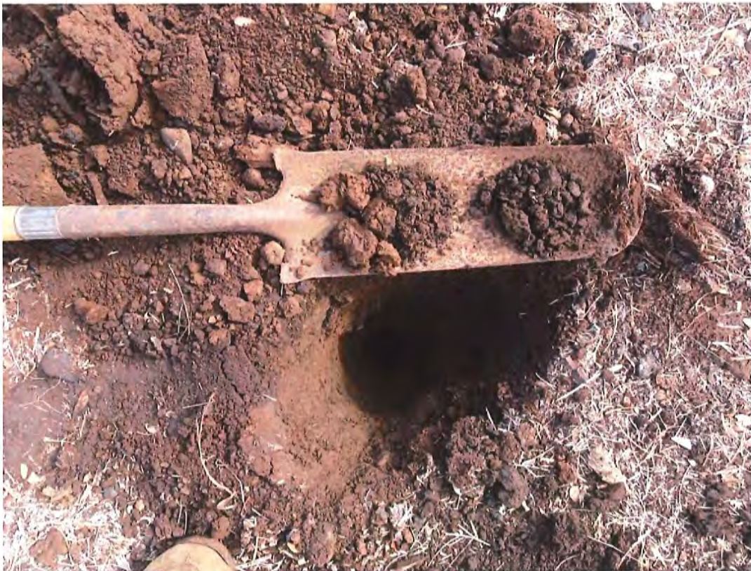
Sampling Point 5B. Dark reddish-brown silt loam over dark reddish-gray clay loam. Saturation at 17 inches. Water table at 20 inches.
