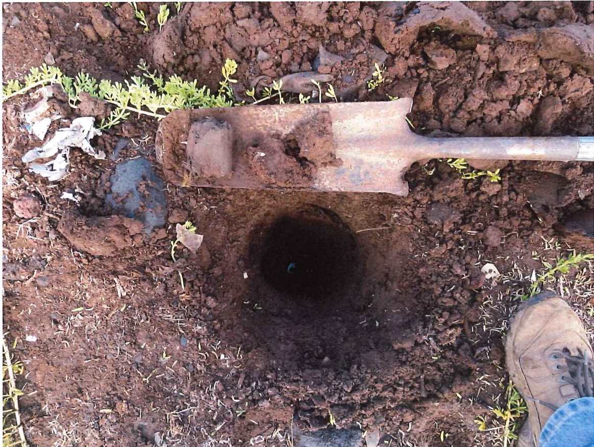
Sampling Point 4B. Dark reddish-brown silt loam over dusky red silty clay loam. Saturation at 19 inches. Water table at 23 inches.
