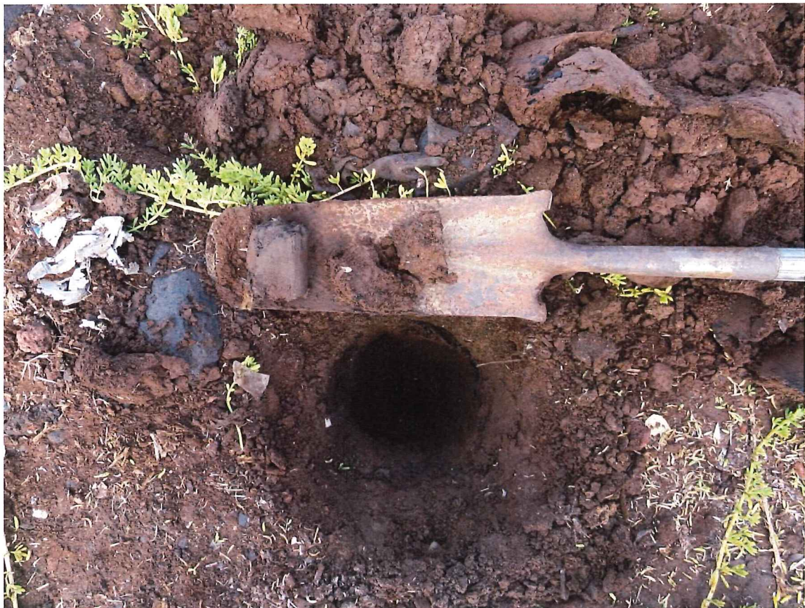
Sampling Point 3B. Dark reddish-brown silt loam over dusky red silty clay loam. Saturation at 17 inches. Water table at 20 inches.
