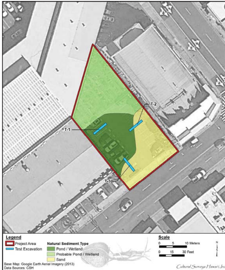
Figure 103. Environmental features (probable pond and sand berm) identified in the project area; suggested extent of pond feature based on testing results and historical documentation of ponds in surrounding property
