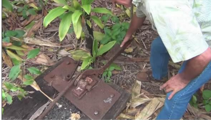
Figure 23: ‘Bush treasure’ repaired ground throw (Courtesy of Scott Johnson)
