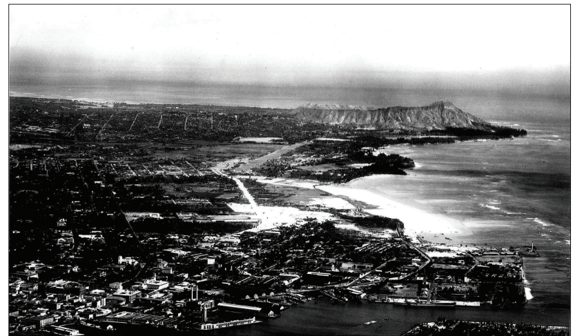
Figure 22. 1931 photograph of the Honolulu to Waikiki Coast; the dredged boat channel and the recent fill for the Ala Moana Regional Park can be clearly seen (Hawai'i State Archives 1931)
