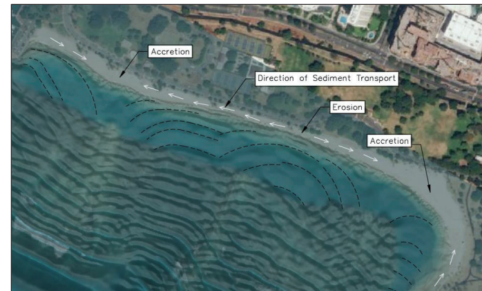
Figure 3-13 Nearshore wave patterns and sediment transport for the modeled prevailing SSW swell
