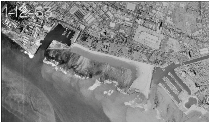
Figure 50. 1963 aerial photograph of the Ala Moana Regional Park with initial construction of the Magic Island peninsula (on right) (UH SOEST 2012d)
