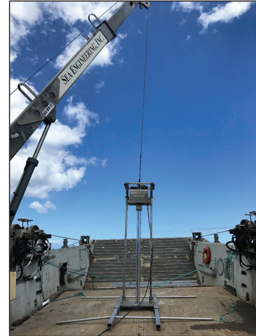
Figure 6-3 Vibracore on the deck of the Huki Pau
