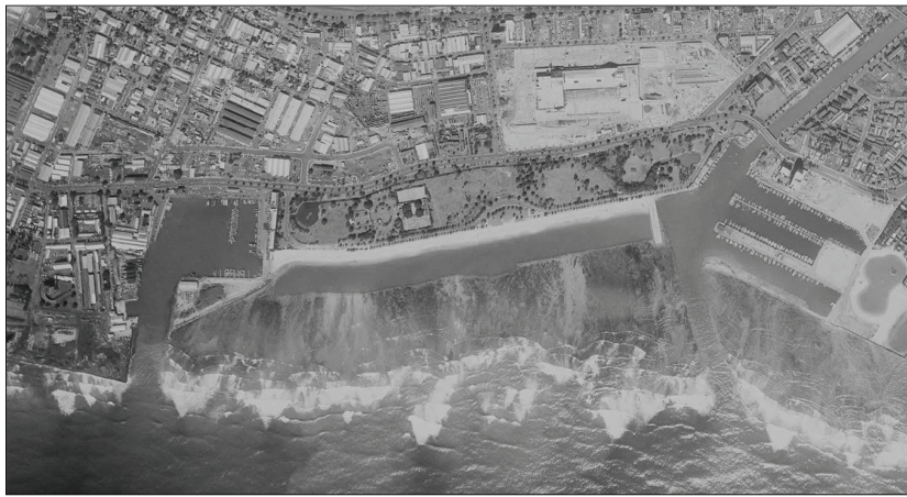
Figure 48. 1959 aerial photograph of Ala Moana Regional Park, with wide beach and swimming area; swimming area blocked from access to Kewalo Basin (left) by peninsula of fill land and from Ala Moana Yacht Harbor (right) by a jetty (UH SOEST 2012c)
