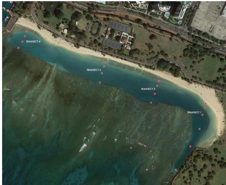
FIGURE 1. Satellite image of Ala Moana Regional Park showing beach, dredged linear swim channel, and undredged reef flat. Also shown are locations of water chemistry sampling stations along four transects that extend from the shoreline to the edge of the dredge cut.
