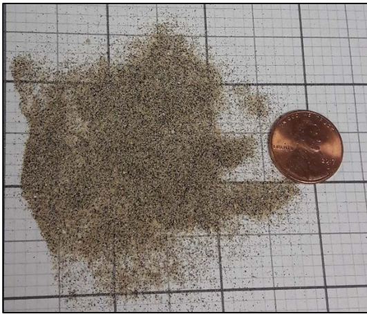
Photo #13: Offshore Sand Sample #2 (farthest sample collected from offshore). Grid size 1/10 inch.
