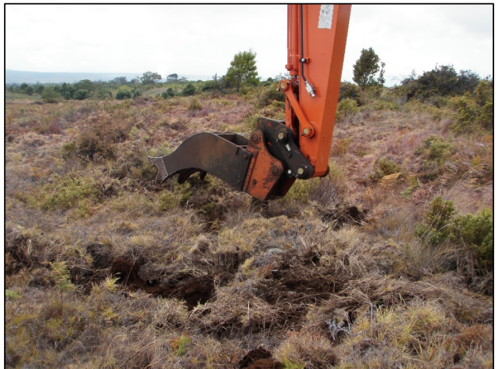
Figure 7. Spot cultivation, using a specialized tool built for the purpose will be used in less accessible terrain and reaching onto steeper slopes. Ripper shank is 3 ft (90 cm) long, proving ample rooting depth early on, improving tree growth vis hand prepared soil which is never able to achieve the depth.
