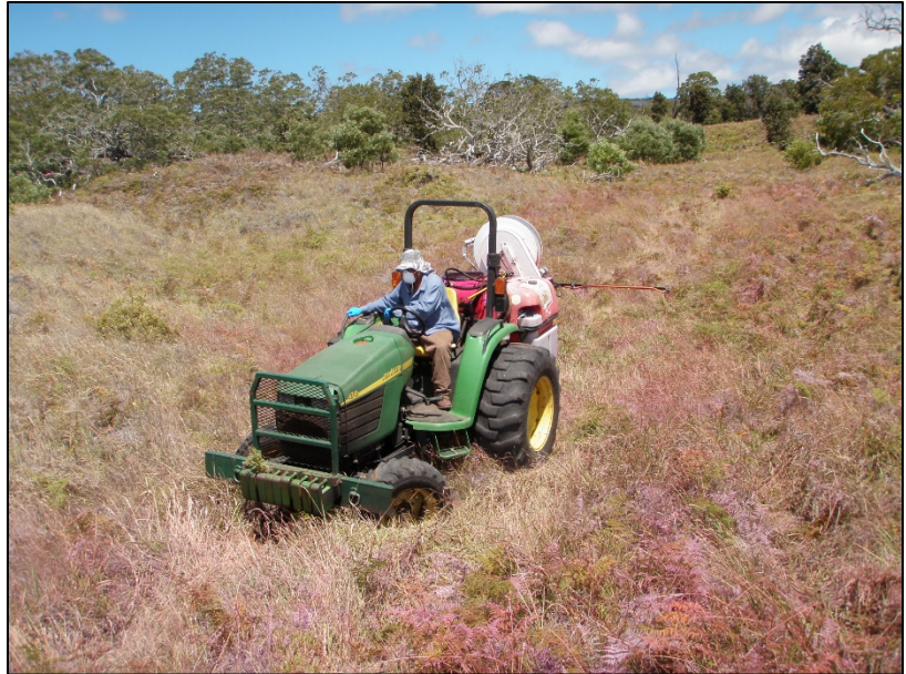
Figure 8. Ground control works very well if the terrain is less than 20% slope, the limit for rubber tire equipment.
