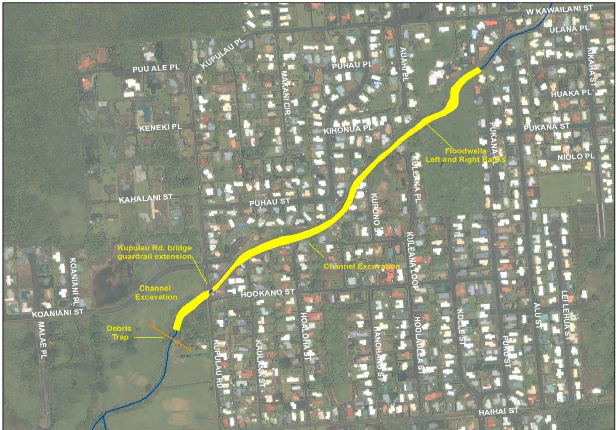
Figure 53. Location of Waiakea Stream Combination of Floodwalls and Channelization
