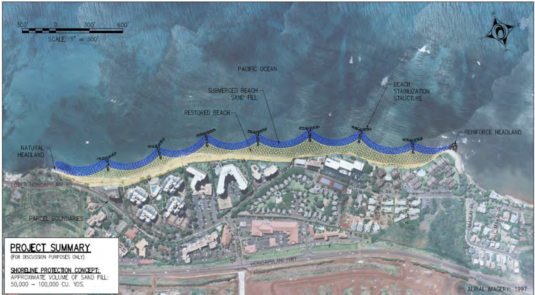
Figure 1-2: Conceptual Sketch of 50,000-100,000 cy Beach Nourishment with Beach Stabilization Structures
