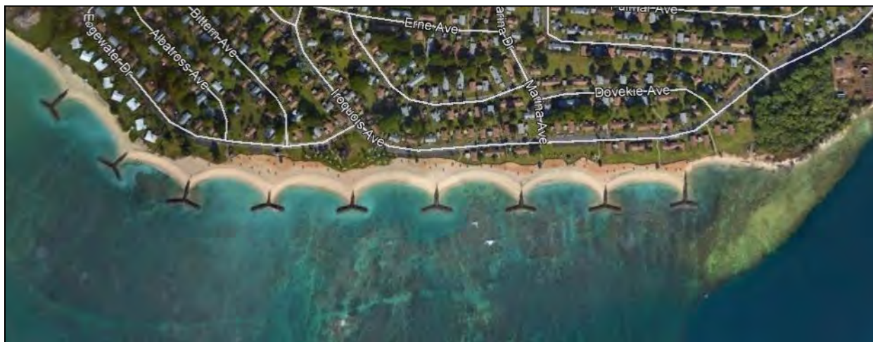
Figure 2-5: T-groins and Nourished Sand at Iroquois Point, O‘ahu, Hawai‘i
