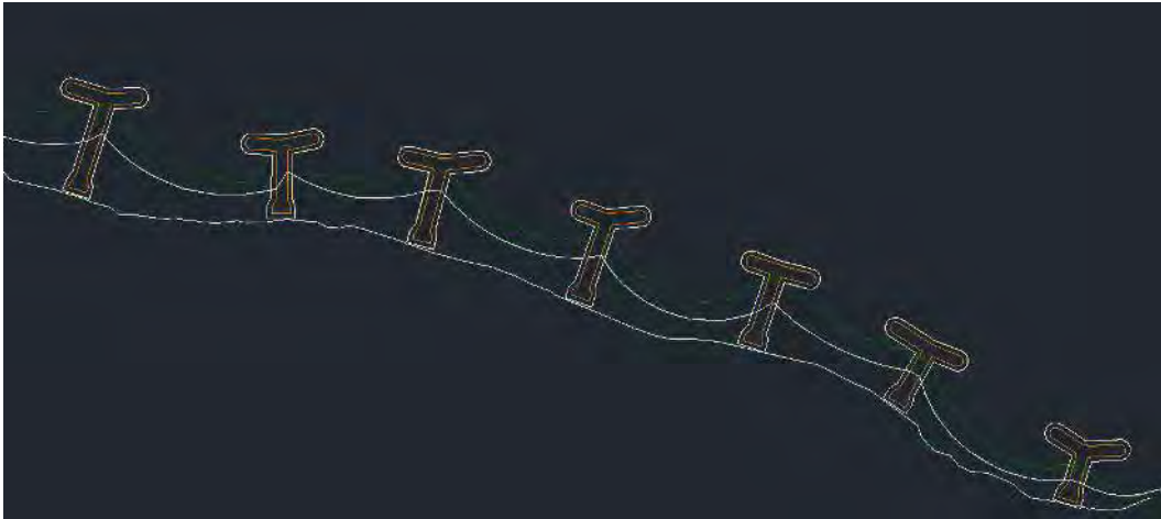
Figure 2: Outlines of the toe and crest perimeters of the seven conceptual groins.
