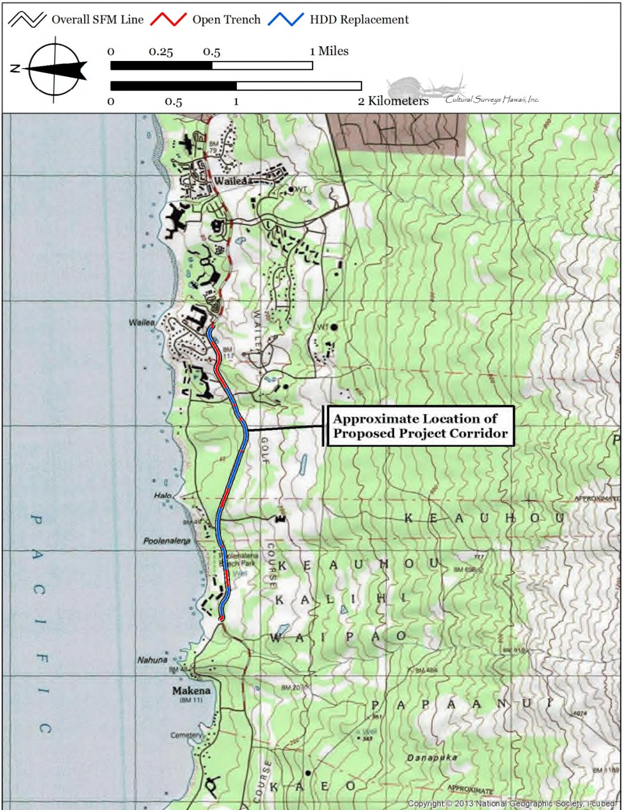
Attachment 1 A portion of the Makena 7.5 minute USGS topographic quadrangle showing proposed Kihei Wastewater Pump Station No. 16 Force Main (SFM) route.
