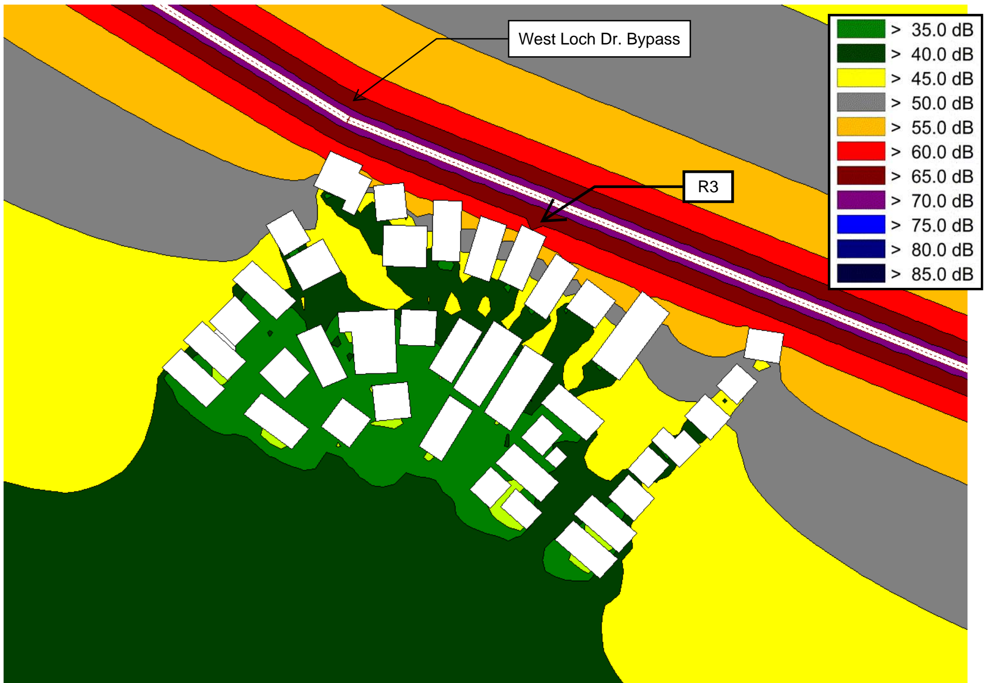
Figure 12. Peak Hour Traffic Average Noise Levels (Leq) at R3 West Loch Drive Bypass Noise Analysis DLAA #18-029 10/26/2018
