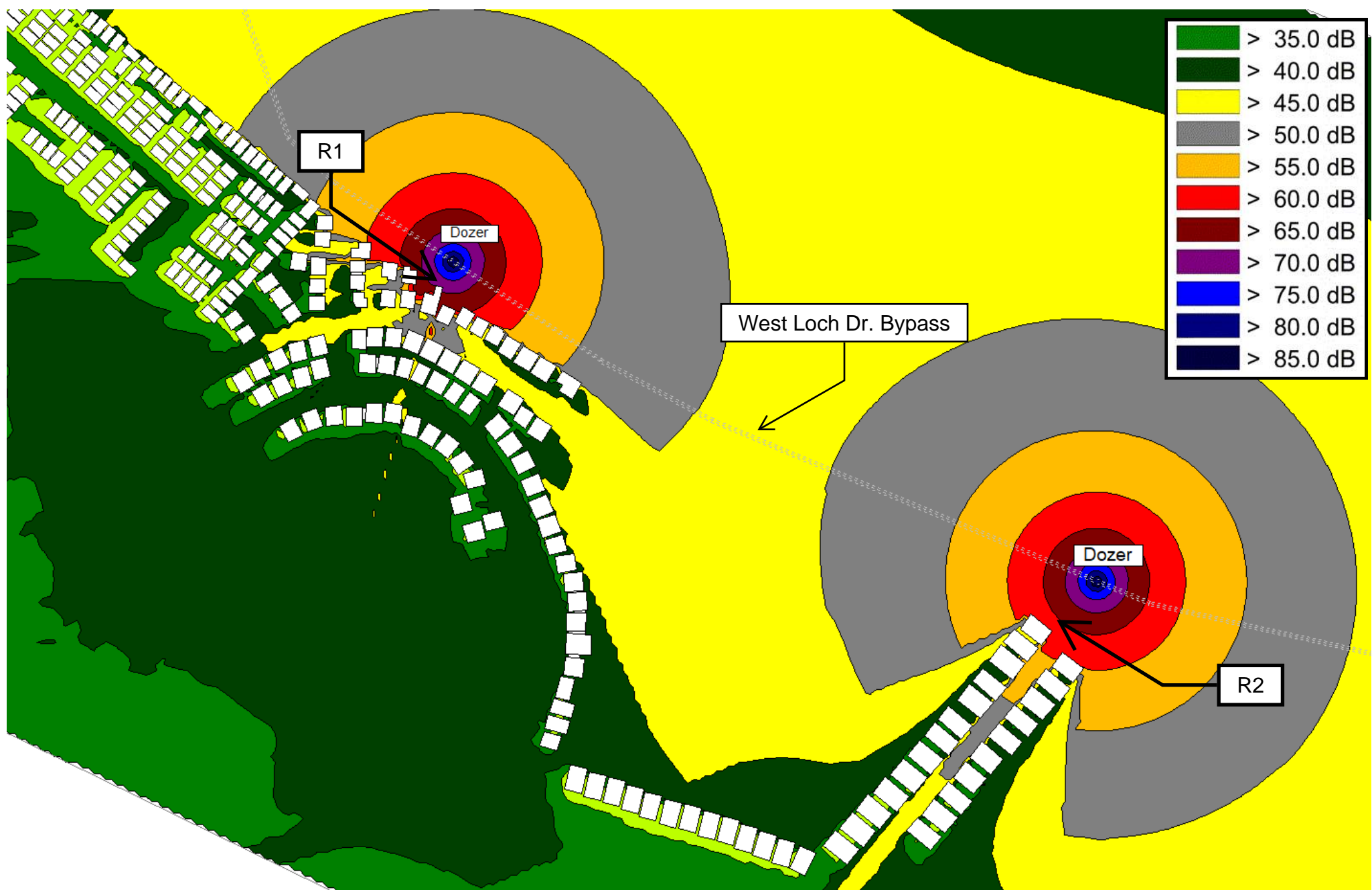
Figure 4. Bulldozer Noise Modeling Results, S1 & S2 Locations West Loch Drive Bypass Noise Analysis DLAA #18-029 10/26/2018
