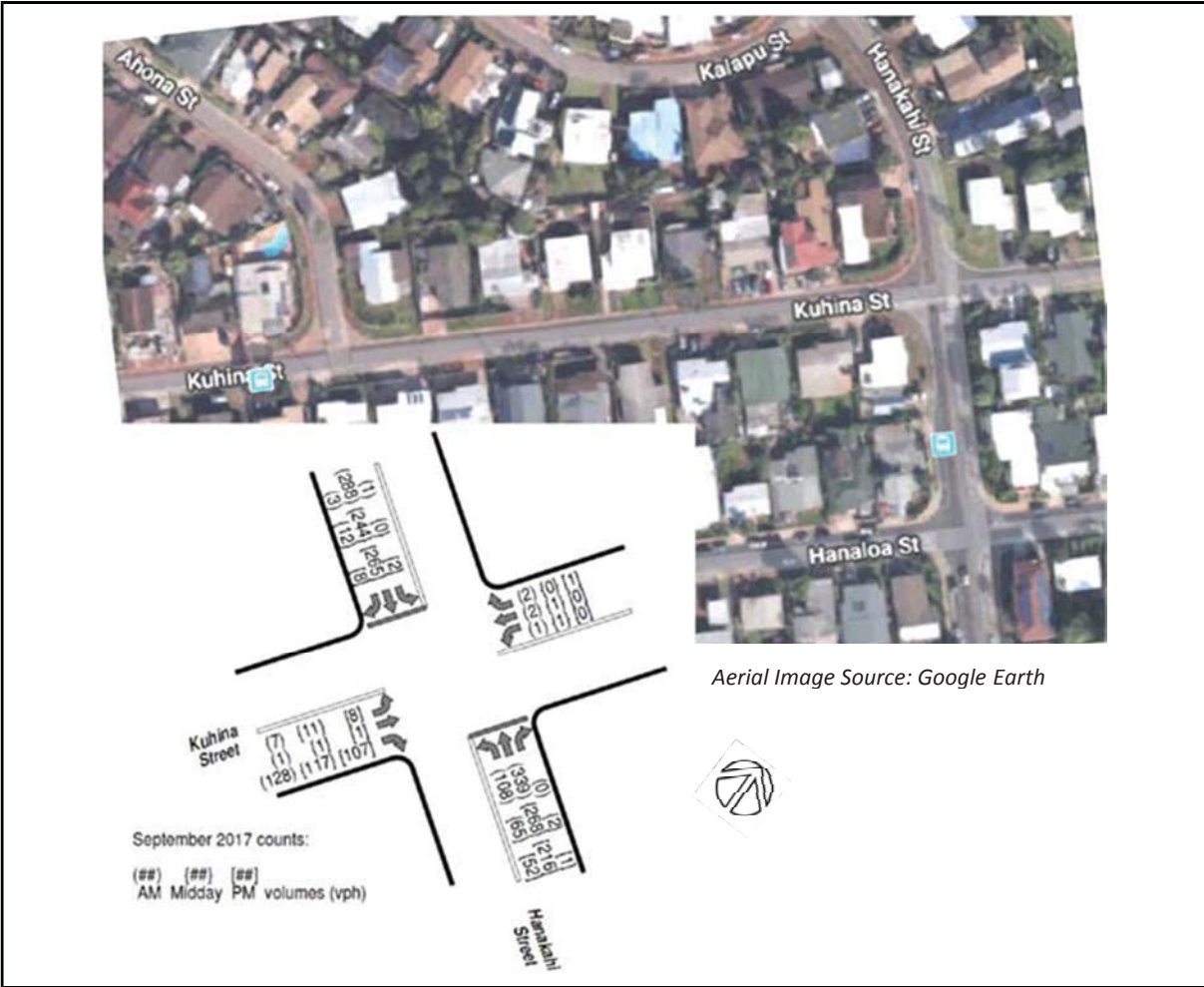
Figure 8 – Intersection 6, Hanakahi Street and Kuhina Street
