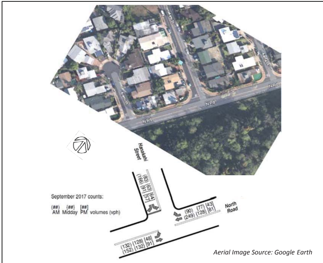
Figure 7 – Intersection 5, North Road and Hanakahi Street
