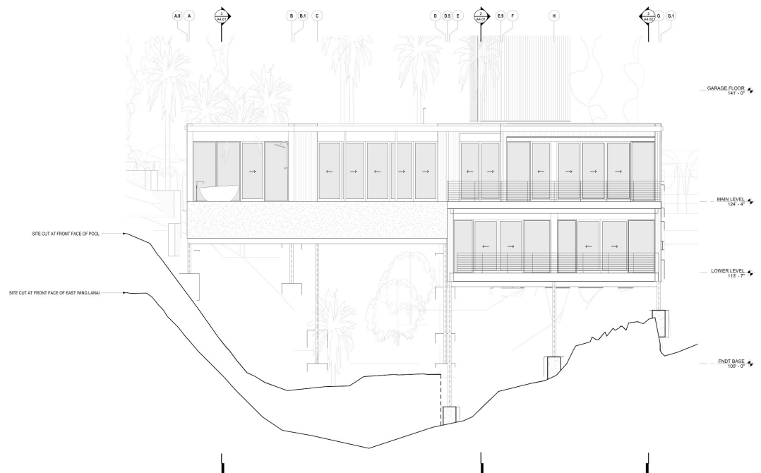
2 SOUTH BUILDING ELEVATION
