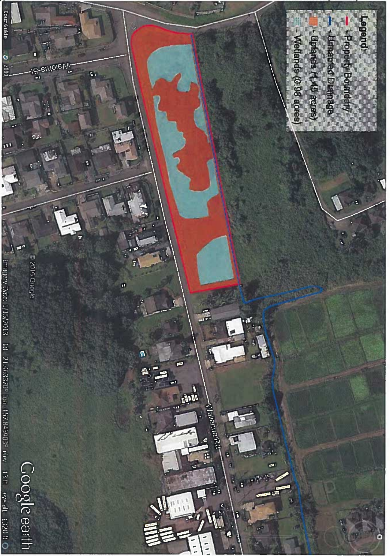
Figure 7: Pre-Fill conditions and resources based on in-office assessment as overlain and quantified in Google Earth
