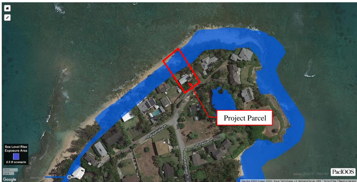
Figure 3.5: Annual High Wave Flooding in Project Area under a 0.5-foot Sea Level Rise Scenario (2030)
