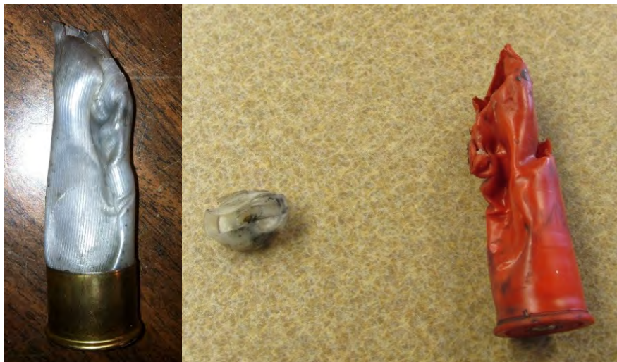
Detonation of ShellCracker inside shotgun barrel results in shell casing melting.
