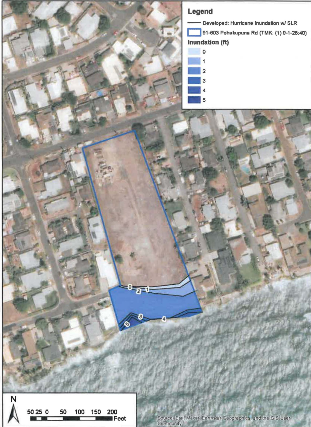
Figure 28. Category 3 Hurricane Inundation for 91-603 Pohakupuna Road Developed Conditions w/ SLR
