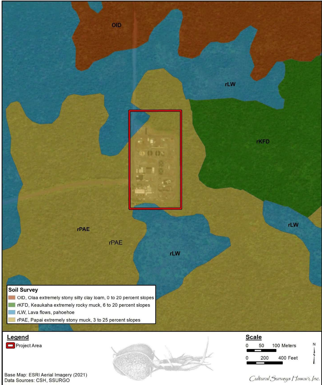
Figure 5. Overlay of Soil Survey of the Island of Hawaii (Sato et al. 1973), indicating soil and land types within project area (USDA SSURGO 2001)
