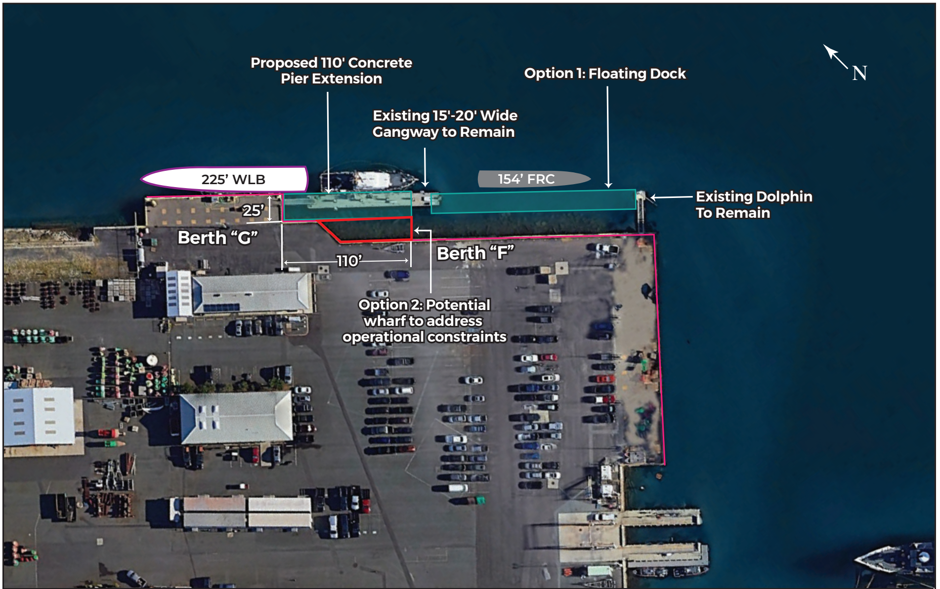
Figure 2: Proposed WLB Mooring and Structural Pier Upgrades
