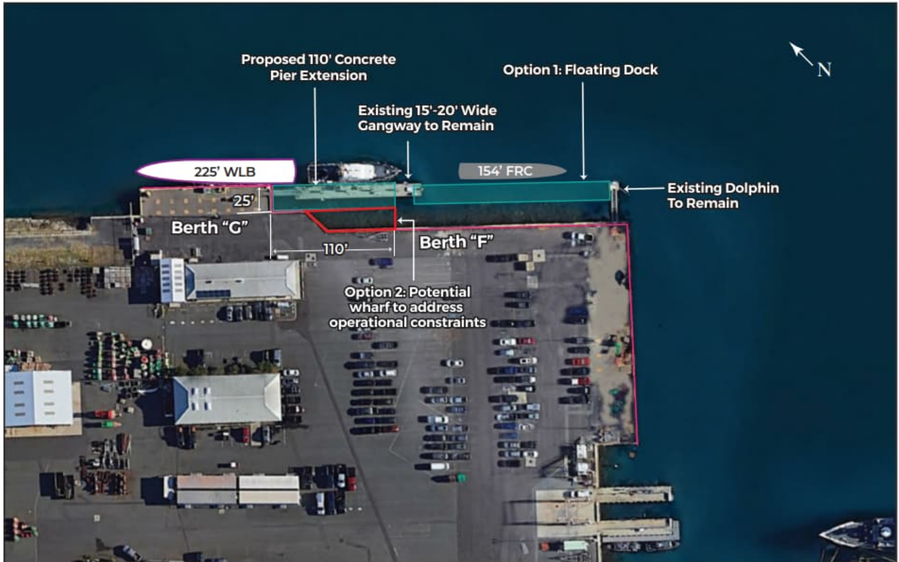
Figure 2: Proposed WLB Mooring and Structural Pier Upgrades
