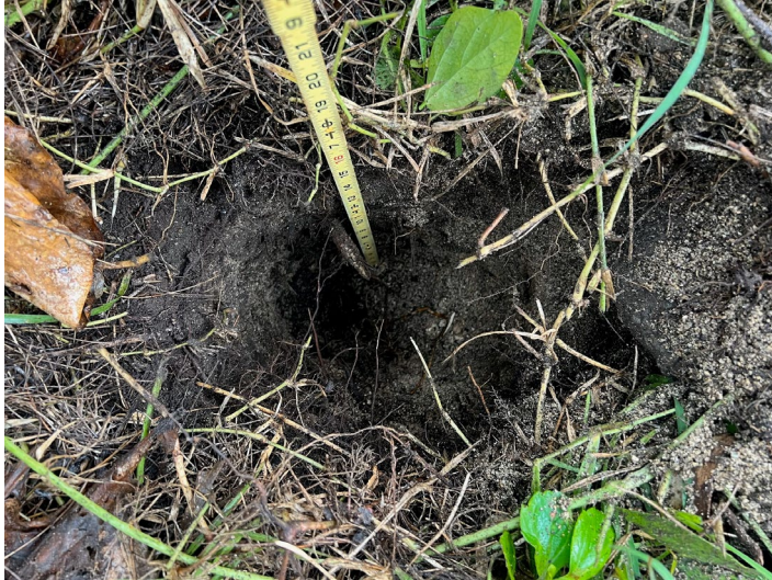
SP-06 is located upland in thick guinea grass ( Megathyrsus maximus ; FAC). Water table is > 13 in deep.
