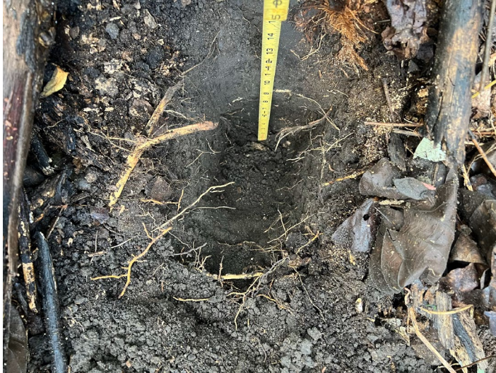
SP-03 is in a cut down hau ( Hibiscus tiliaceus ; FACW) forest. Water table is > 15 in deep. Surface water is ~5 m away.
