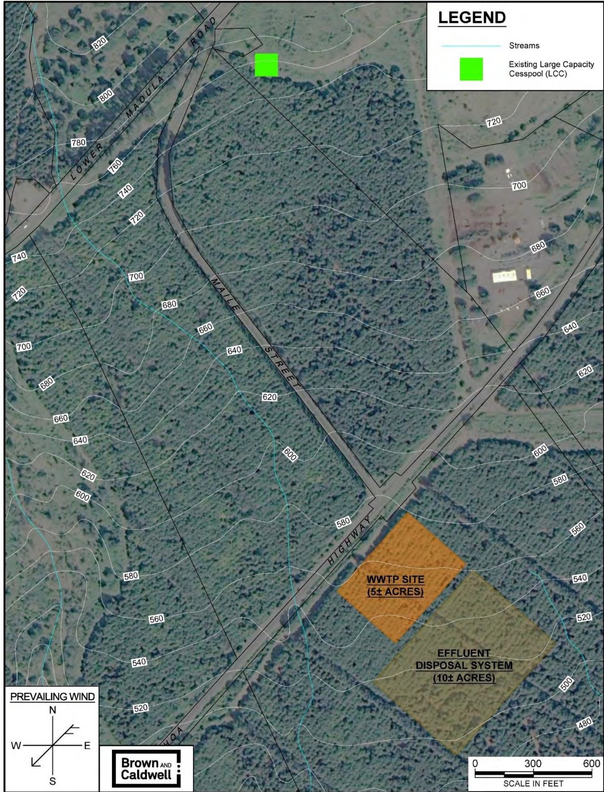
Figure 2.8. Site 9 Alternative – Preliminary Site Plan for New Wastewater Treatment and Disposal Facility
