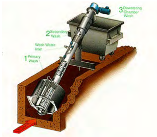
Figure 5: In-Channel Cylindrical Screen Source: PER, 2023
