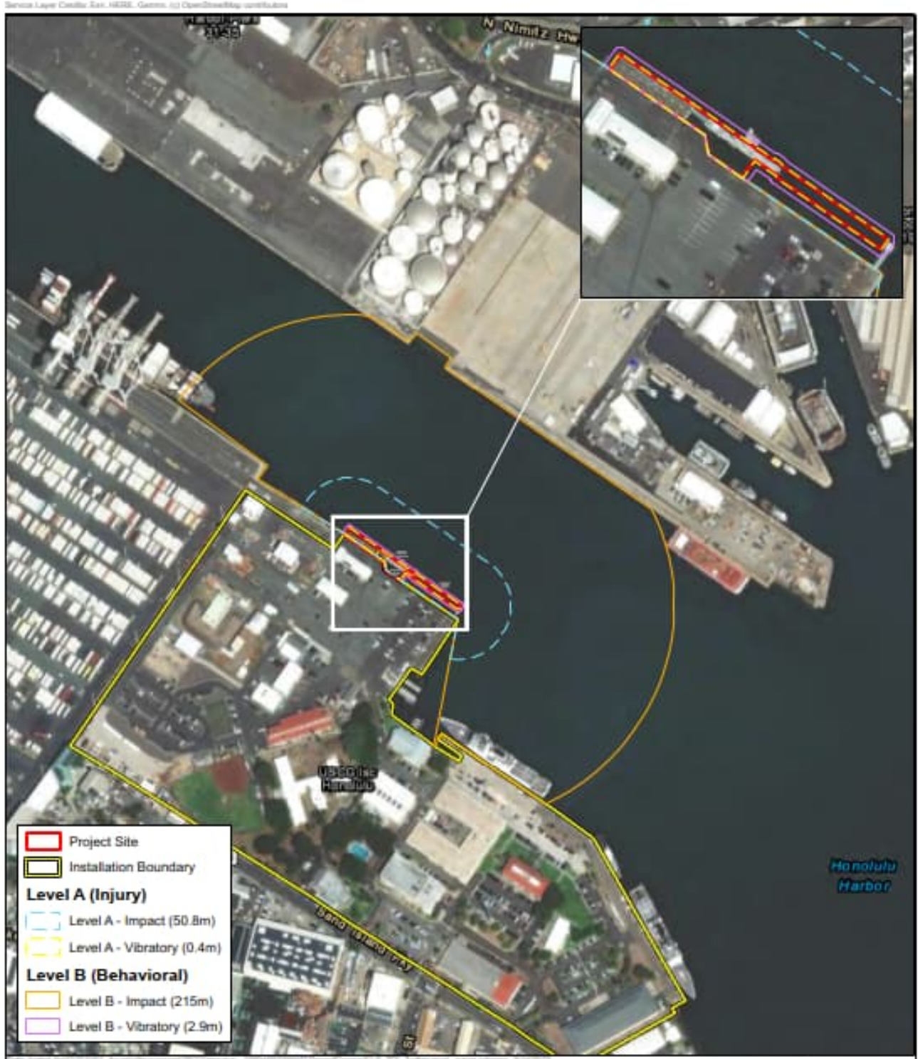
Figure 4: Level A (Injury) and Level B (Behavioral) Zones For Green and Hawksbill Sea Turtles WLB Mooring and Structural Pier Upgrades
