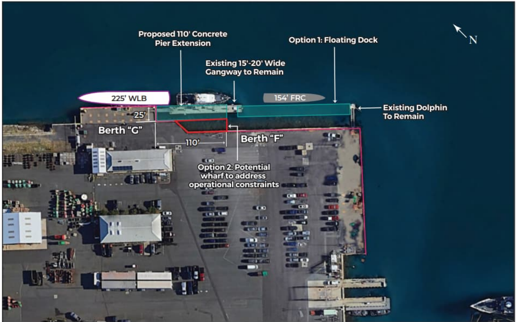
Figure 2: Proposed WLB Mooring and Structural Pier Upgrades
