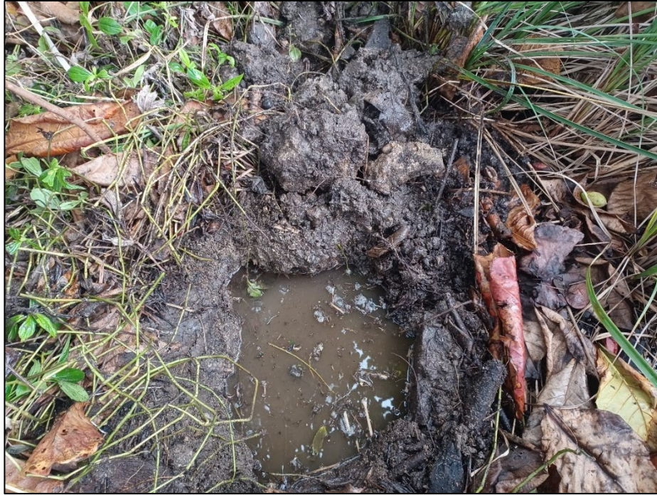
Figure 8. The soil at SP-02 is a sandy clay loam at the surface, and muck matrix (hydric, A8) with 80% asphalt below 6 in. The water table is 4 in below the surface.
