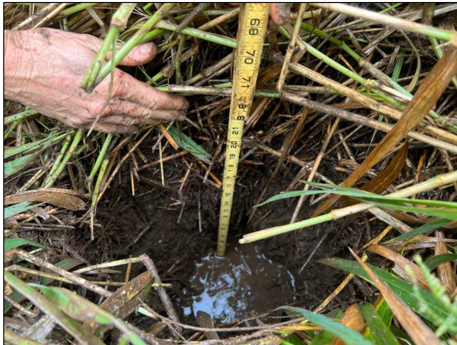
Figure 7. A high groundwater table (shown here at SP-04 at 12 in below the ground surface) is the primary source of wetland hydrology for the subject wetland.
