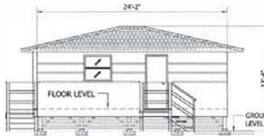
3 EXIST. RIGHT ELEVATION 3/16" = 1'-0"
