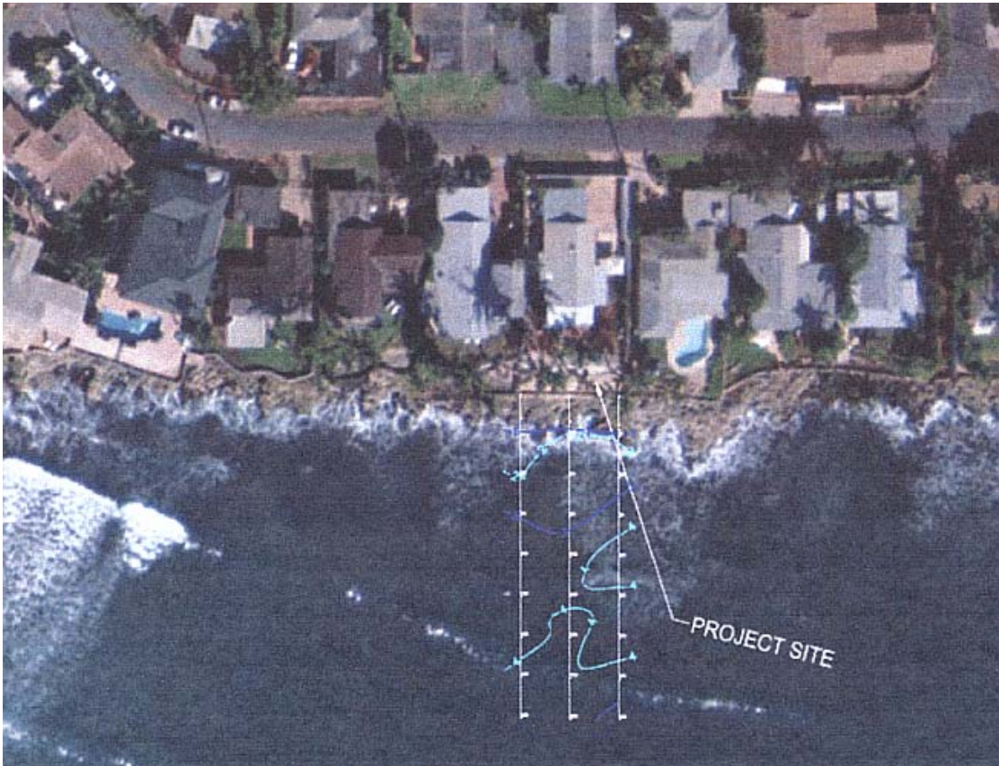
Aerial photo of project site with offshore bathymetry (survey lines are 200 ft) (photo courtesy of UH Coastal Geology Group Website)
