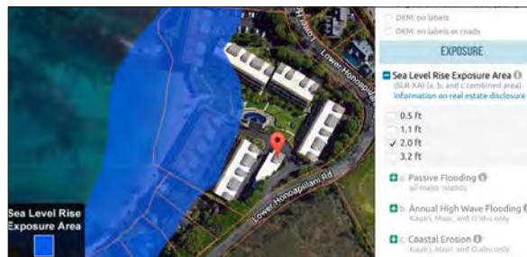
2.0 feet exposure SLR-XA line Kahana Sunset's Building A and Building F, and a portion of Building B and Building E and common area are located within the hazard line
