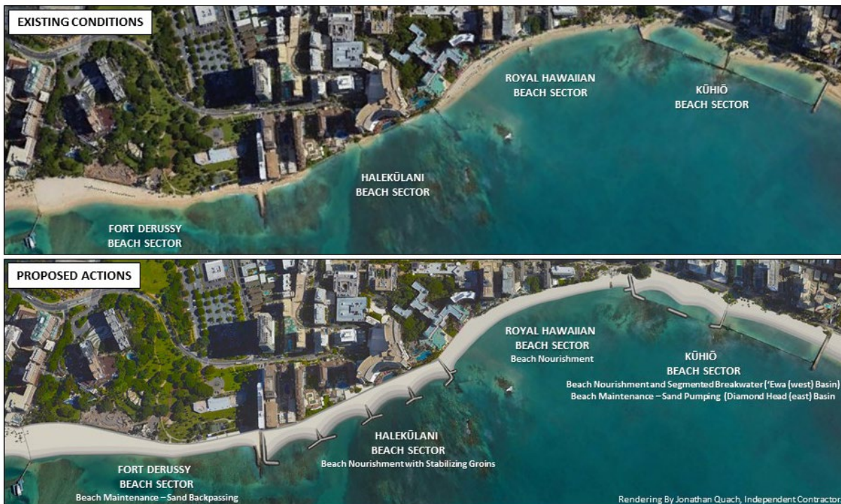
Figure A3-3. Conceptual rendering of proposed beach improvements at Waikīkī, O'ahu
