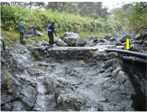
View upstream at next diversion from previous site gh063r-040208. Note 6" black PVC pipe (yellow arrow) on the right which is diverting water from the stream channel and carrying it downstream. Upper reach Pi'ina'au Stream, Maui, Hawai'i.
