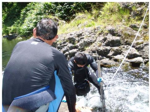
Figure 4-8. Photo of the flow measurement near survey site 1. (6/30/2009; Tributary name: Hanawī (64022001); PBN: sh001p-058-063009; Surveyor: Hau, S.; SBN: 124; Lat. (DD): 20.81592, Long. (DD): -156.10379).
