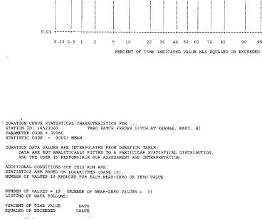
LOG-NORMAL DURATION PLOT FOR PERIOD OCT TO SEP STATION ID: 16522000 TARO PATCH FEEDER DITCH AT KEANAE, MAUI, HI PRANMETER CODE - 00060 DISCHARGE STATISTIC CODE - 00003 MEAN
