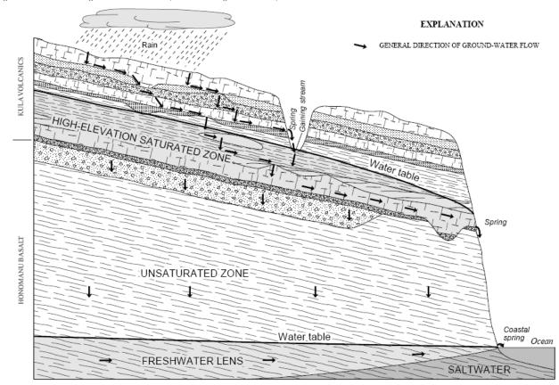
**Figure 3-1.** Diagram illustrating the ground water system west of Keanae Valley, northeast Maui, Hawaii. Arrows indicate general direction of ground water flow (Source: Gingerich, 1999).
