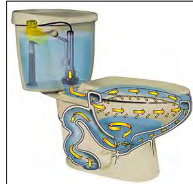
Gravity Flush Toilet Flow Schematic
